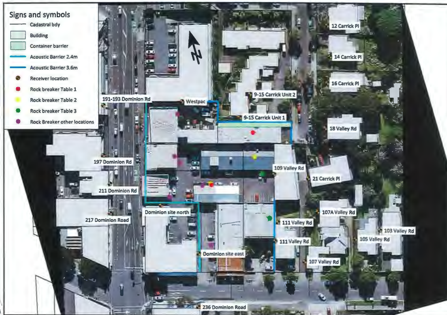
Figure 1 – rock breaker, receiver and barrier locations used for noise modelling
